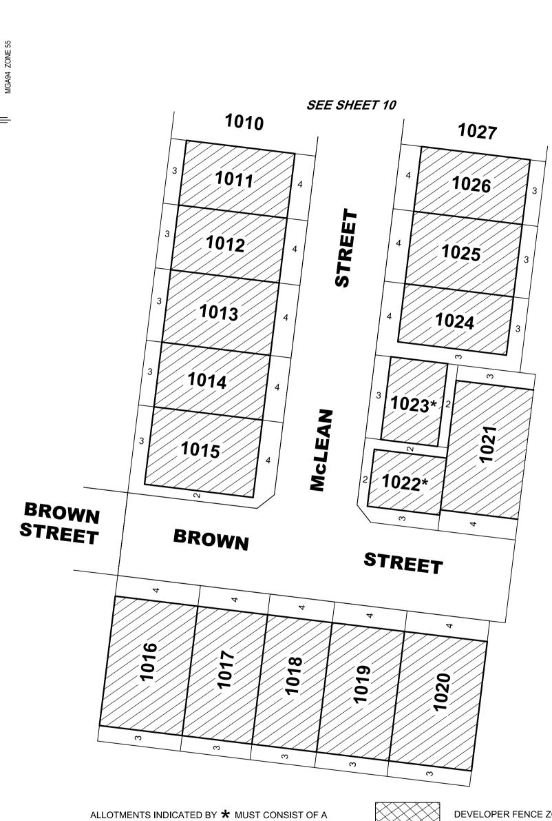
SECLUDED PRIVATE OPEN SPACE WITH A MINIMUM AREA OF 25m<sup>2</sup> AND A MINIMUM DIMENSION OF 4 METRES AT THE SIDE OR REAR OF THE DWELLING WITH CONVENIENT ACCESS FROM A LIVING AREA. GARAGES MUST BE SETBACK 5.5m FROM THE FRONT BOUNDARY, NOT EXCEEDING A LENGTH OF 6.5m WHEN CONSTRUCTED ON A BOUNDARY.
